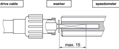
The length of the square above the washer mustn't exceed 15mm and must be shortened and burred if needed. Please note that the cable inside the drive cable may move, for example by the steering angle. Fix the lock nut hand-tight.
